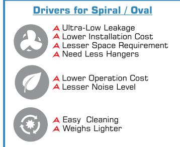
The big commercial advantage is the perimeter of round ducting system is less by 20% or more of same cross section of rectangular ducting. The area of ducting and insulation is less by the same percentage.
